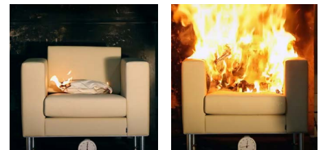
DIN 66084 test, demonstrating a failed product
