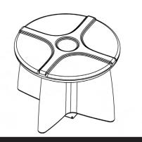
Set product into required position and mark off the center of each position to be drilled through the fixing plate
