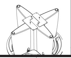
Position fixing plate over the threaded inserts on the bottom of the table so that the countersunk holes are in line with the inserts. Using your fingers, screw the bolts through the plate and into each insert
