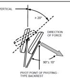
Test has been performed pushing the backrest backwards
