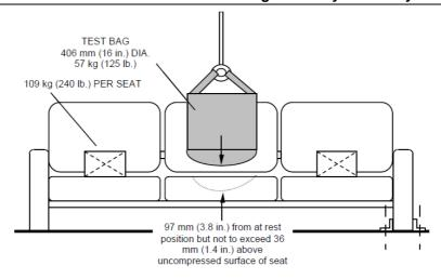
Minimum thickness of cushiony materials of seat: > 50 mm Thickness of additional foam: 0 mm (IFD al 25% di 200 N  $\pm$  22 N)
