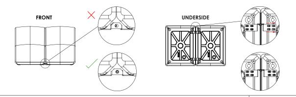
Note: If the securing holes on the brackets are misaligned, unscrew the x4 M6 security bolts that are holding the misaligned bracket in place until the bracket becomes adjustable.
