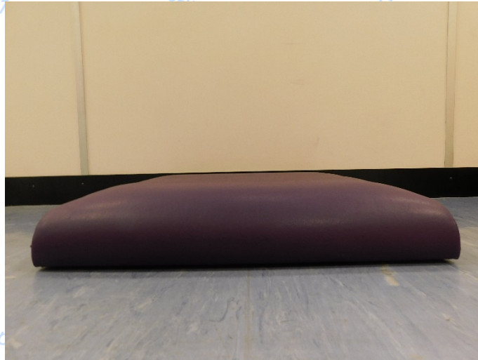
Photo 1: Showing 'Seat cushion 1 – 25mm lilac foam and purple fabric' at 0 cycles
