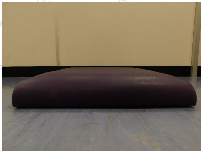
Photo 2: Showing 'Seat cushion 1 – 25mm lilac foam and purple fabric' at 80,000 cycles
